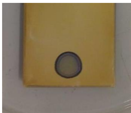
Fig. 21 Double “coffee-ring” formed over AgI@Au of a BV1 extraction
