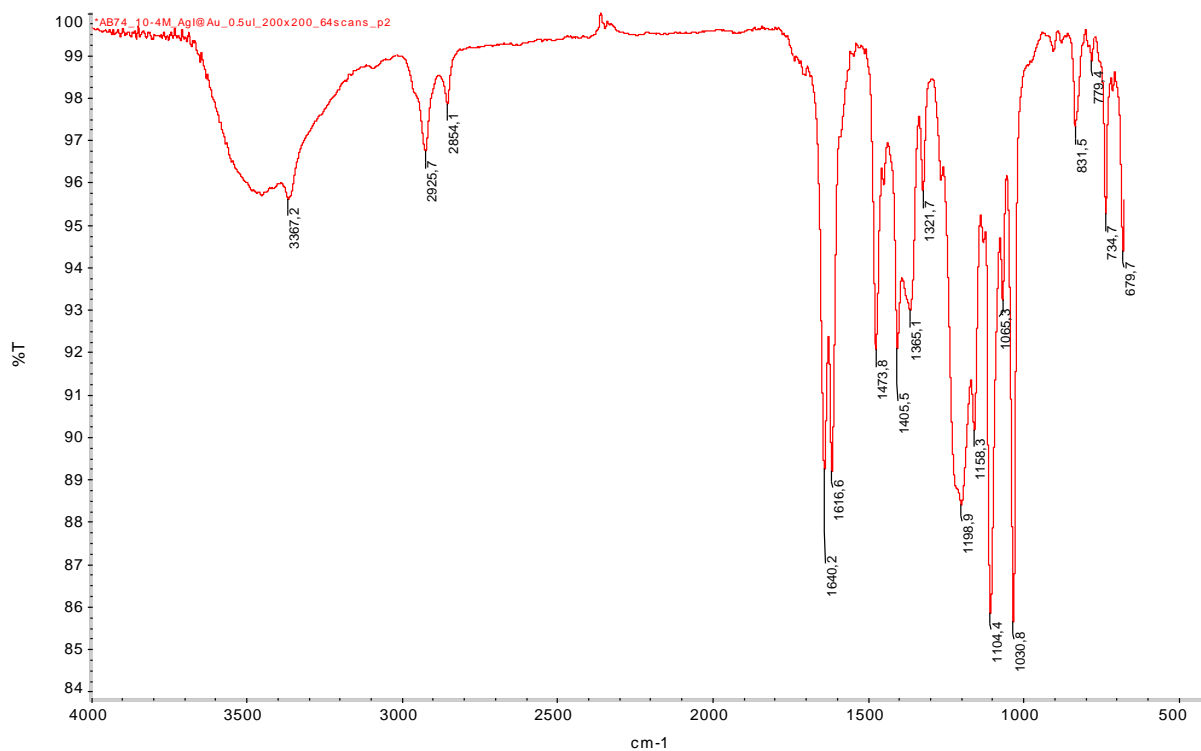
Fig. 3 FTIR spectra of AB9 standard solution 10^{-4} M
