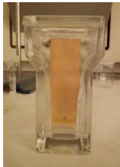
Fig. 9 TLC chamber used for the separation.
