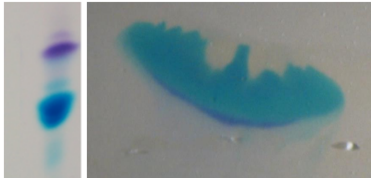
Fig. 50 TLC results of Stabilo® 68/41 analysis. At the left, the results obtained by D'Ambrosio using Si plates, at right the results obtained with the AgI@Au system.
