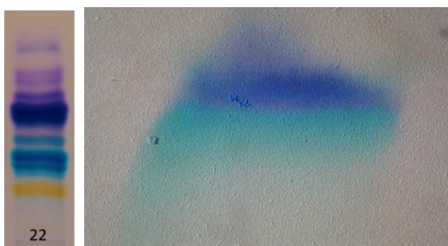
Fig. 44 TLC results of 68/22 Stabilo® ink. At left is shown the results obtained by D'Ambrosio, at right are the results using AgI@Au plates, 2.5x.
