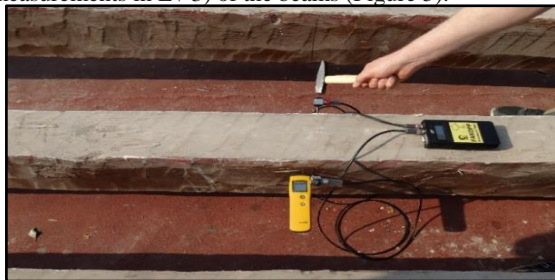
Figure 5. Measurements of the humidity content and wave velocity.
