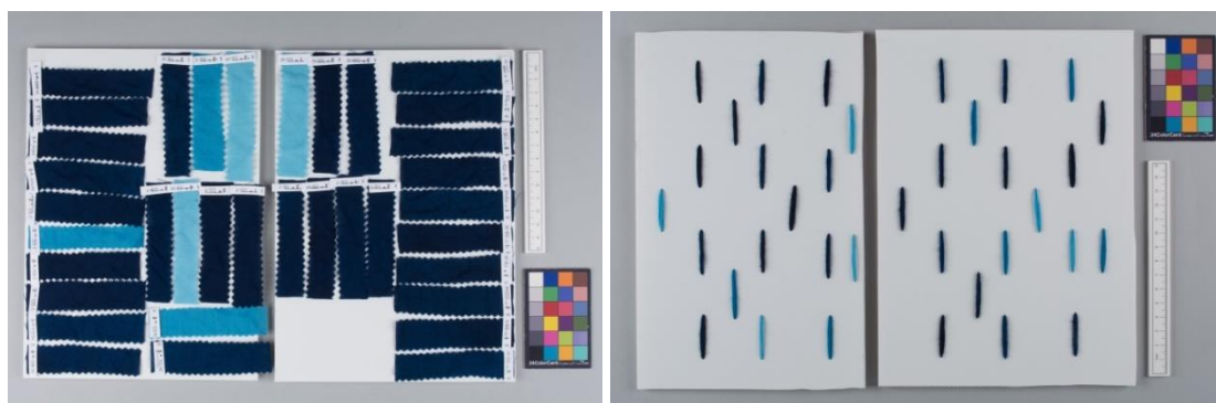
Figures 4.11 and 4.12. Fabric tray (left) and thread tray (right) for artificial ageing © CTCTAH, University of Glasgow, 2018. Photos by author.
