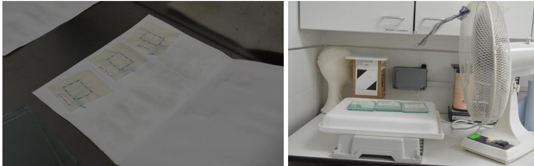
Figures 5.2 and 5.3. Drying process of embroidered fabric samples by absorption with blotting paper (Group B)(left) and by air circulation with a fan (Group H)(right). © CTCTAH, University of Glasgow, 2018. Photos by author.
