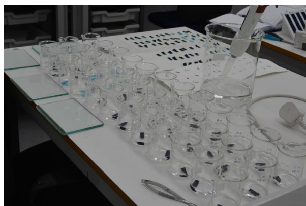
Figure 6.5. Beakers test to evaluate dye solubilisation © CTCTAH, University of Glasgow, 2018. Photo by author.
