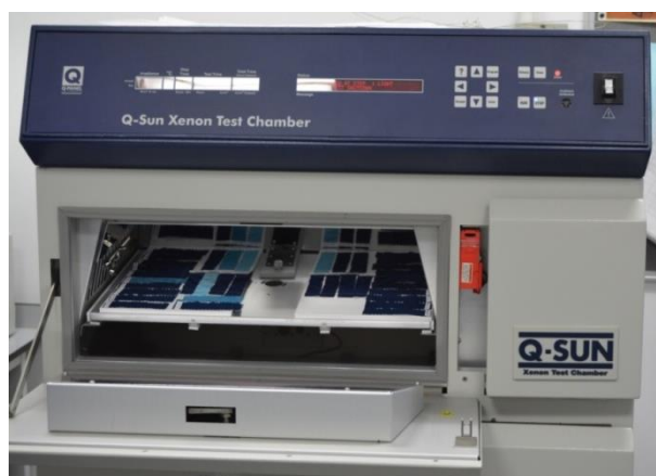
Figure 1. Q-Sun Xe1 Xenon Test Chamber with fabric tray on the inside
