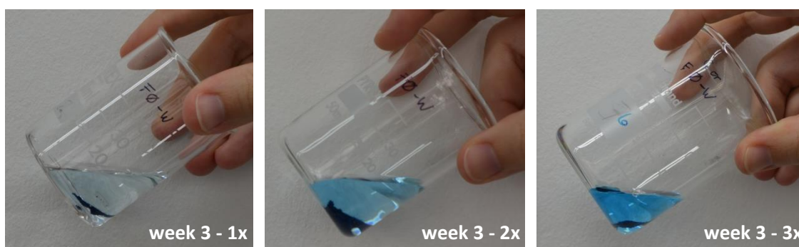
Figure 6.13. Washfastness results (beakers test) after repeated wetting and drying cycles for non-mordanted sample, dyed with Fisher indigo carmine at 45-50 °C ( F0-W ) from the storeroom scenario after week 3. The visibility of solubilised dye increased after each cycle.
