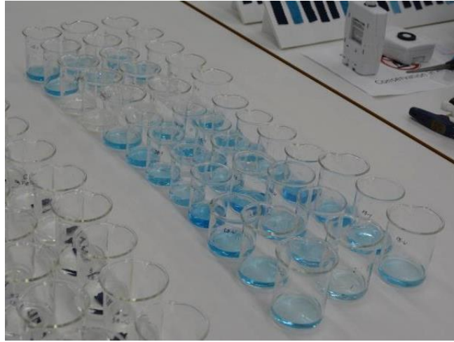
Figure 6.15. Beakers test showing positive results for solubilised dye on most samples, throughout additional testing. © CTCTAH, University of Glasgow, Photo by author.
