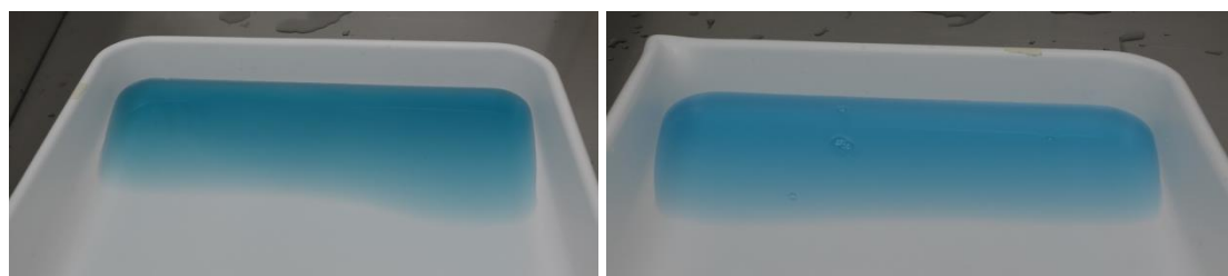
Figures 7.7 and 7.8. Solubilised dye from Sampler 1808 after first (left) and second rinse (right) © CTCTAH, University of Glasgow, 2018. Photos by author.
