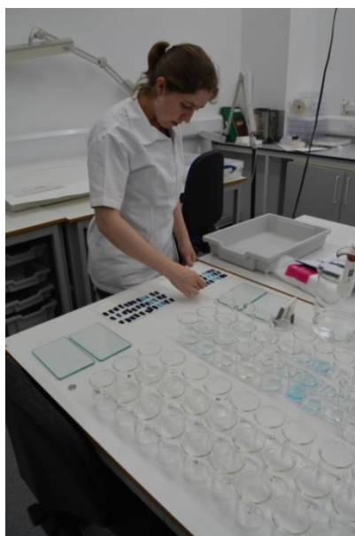
Figure 6.9. Repeated drying and wetting cycles of fabric samples to test washfastness © CTCTAH, University of Glasgow, Photo by Megan Creamer.
