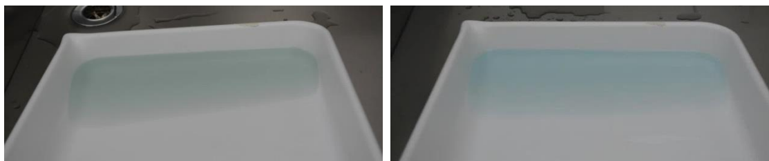
Figures 7.5 and 7.6. Solubilised dye from Sampler 1783 after first (left) and second rinse (right) © CTCTAH, University of Glasgow, 2018. Photos by author.
