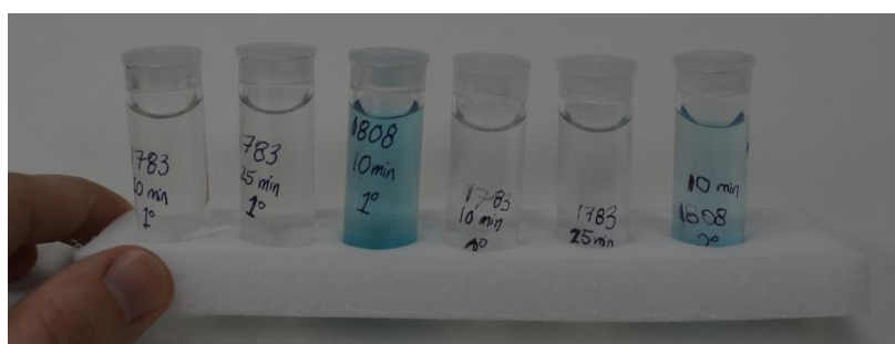
Figure 7.4. Collected samples of solubilised dye per rinsing cycle © CTCTAH, University of Glasgow, 2018. Photo by author.
